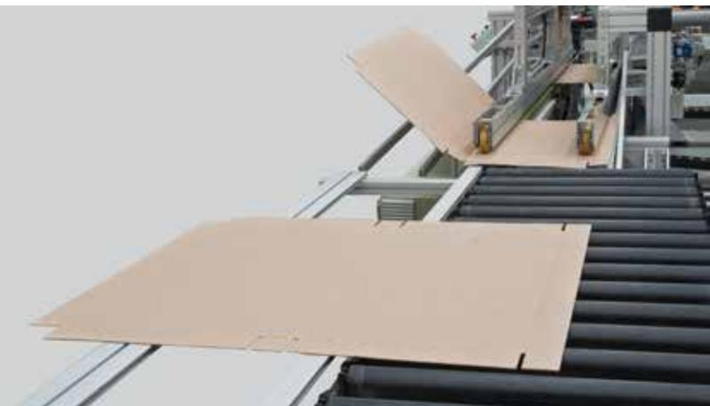
This line has been designed for erecting boxes Mod. FEFCO410. The longitudinal flaps are folded within the first station while the transversal ones (2) are glued and folded with hot-melt glue in order to form the basic "tray" within the second station.
